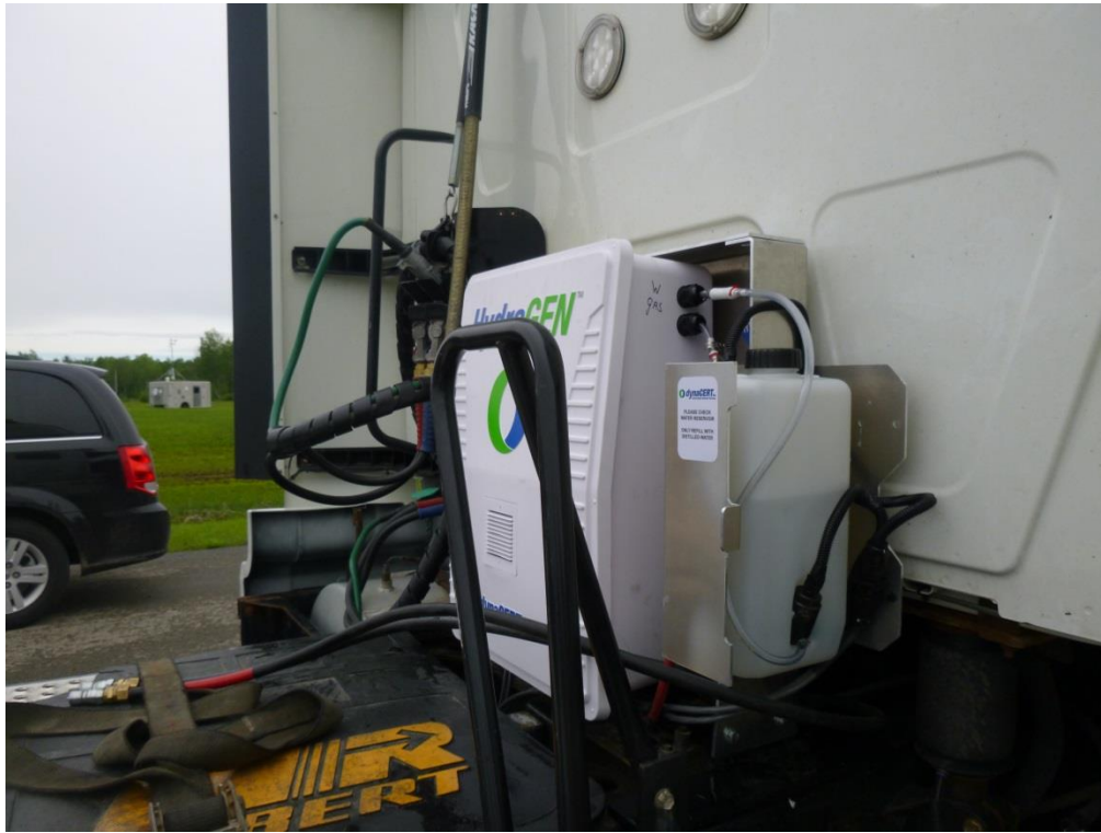
Figure 6. Installation of HydraGen™ on test vehicle C6 (2243).
