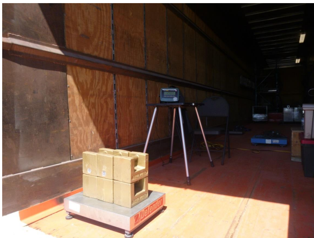
Figure 13. Scale checking using a calibration weight set.
