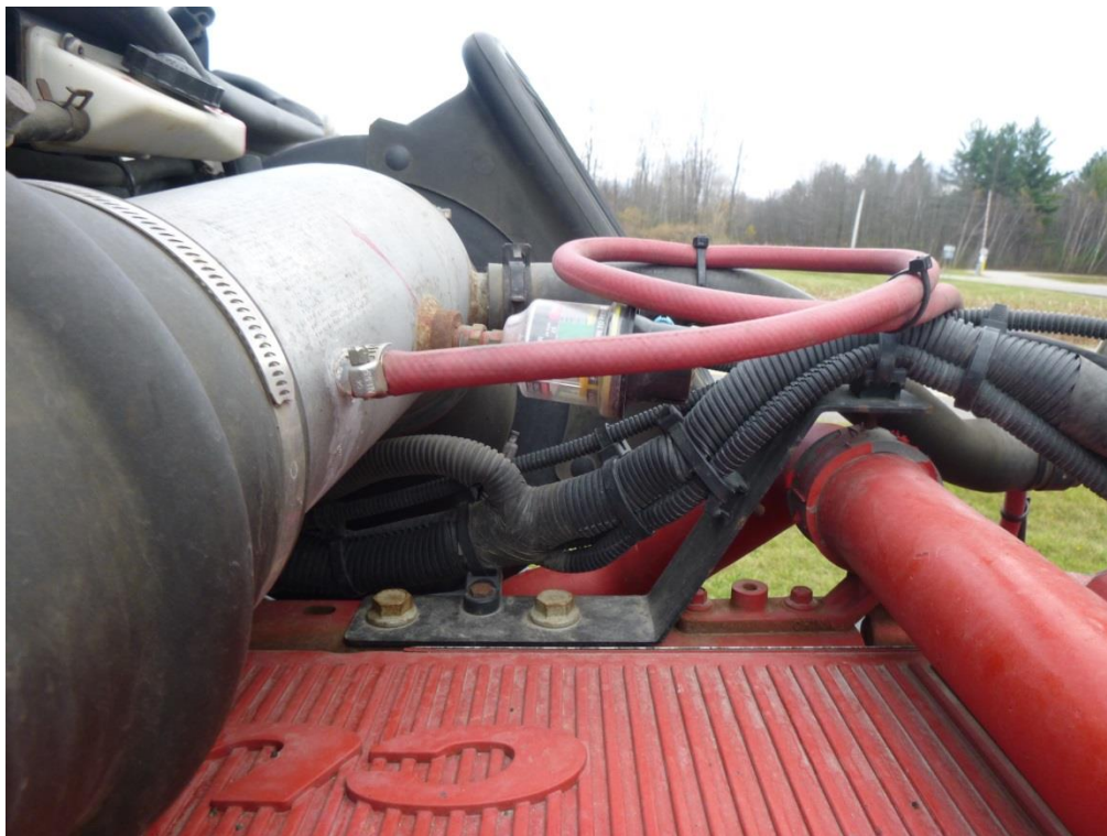
Figure 7. Gas injection port on air intake manifold on test vehicle C6 (2243).
